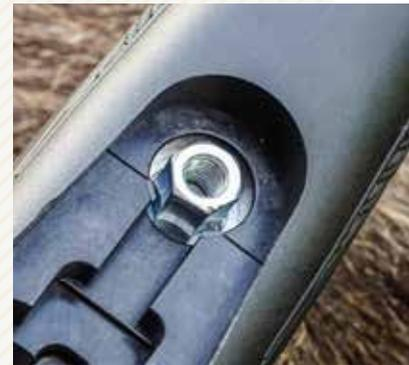
▲ *The recessed 10mm nut tightens up on the front action bolt but given the minimal clearance it's not easy to find a socket that will fit.*
