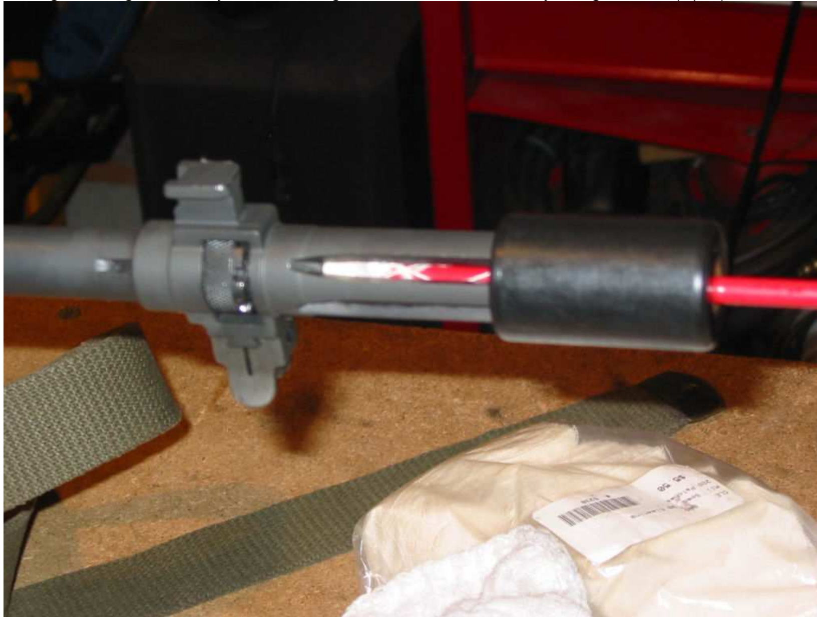
7. Using the bore guide to safely run the cleaning rod and its attachments safely through the bore (2 pics)
