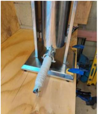
**Step 6**, fill up the stuffing machine. This is just a big cylinder with a piston in it. A wee valve lets air out top so the sausages don't end up with too many voids. I have yet to work out a better way than loading the raw mixture in by the handful. It's a messy step. The one I have is a 7 litre capacity vertical arrangement. There's a gear box that drives the piston down into the cylinder. It cost me around \$400. The single most expensive part of the job.
