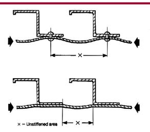
Fig.1 Stiffening effect - bonding and riveting compared
