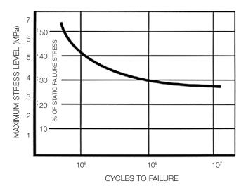
Fig.11 Fatigue strength (tensile) of lap joints
