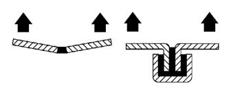
Weak cleavage joints can be strengthened through design, in this instance by adding a U-section to the previously bent sheet.
