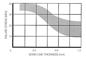
Fig.10 Bond-line thickness vs. shear strength
