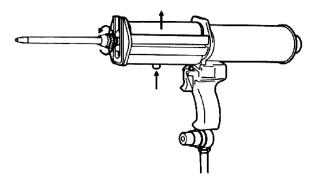
Fig.15 Handgun operated by compressed air
