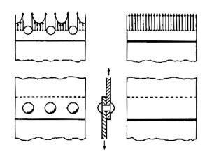
Fig. 2 Stress distribution in loaded joints
